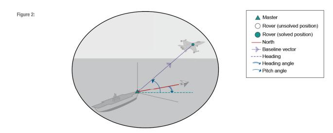
Figure 2 illustrates the Master receiver located on a marine vessel and the Rover receiver located on a fighter jet. Relative heading, pitch, baseline length and Rover positions are computed with respect to the Master receiver.
