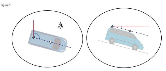
Figure 1 illustrates Master and Rover receivers located on the same vehicle and two antennas installed at a fixed distance from one another. Relative heading and pitch are computed with respect to the Master receiver.
